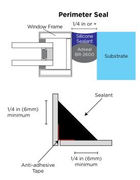
When it is not possible to use a conventional backer rod (ADSEAL BACKER ROD), it is recommended to use an anti adhesive tape.
